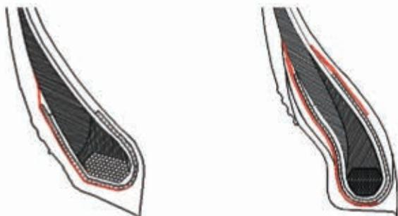
Design of tubeless type tire bead reinforced
