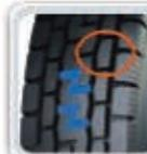
■ Design of big ratio for block and grooves improves tire's abrasion resistance;
